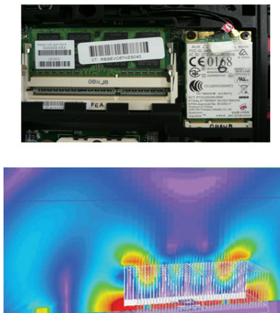
Fig. 47. RF module location and nearby field distribution.
