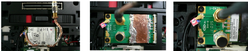
Fig. 49. Circuit ground and chassis ground.
