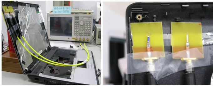
Fig. 36. Placement of two chip antennas insidemold.
